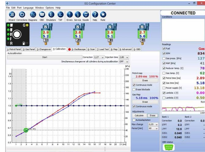
1 Go for a test drive to collect gas map (blue colour) in full range of loads (drive until 100% of map will be collected).
