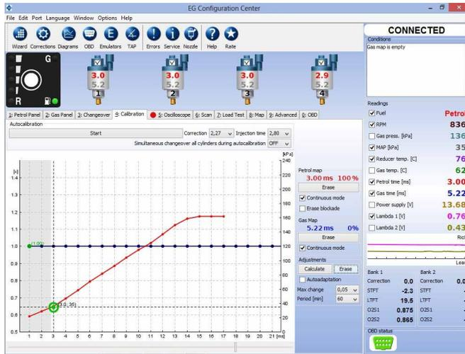
1 Go for a test drive to collect petrol map (red colour) in full range of loads (drive until 100% of map will be collected).
