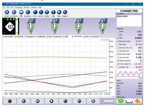
Oscilloscope shows run of selected ECU signals. On the right side of main window we can select (by marking a tick) which ECU signals we would like to see on oscilloscope run. We can also visualize required OBD readouts by selecting them from OBD icon located on the left side of the Toolbar.
