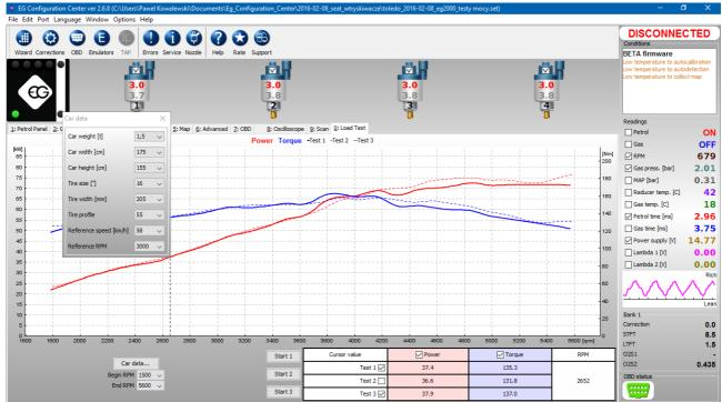
We should select gear 3<sup>rd</sup> and accelerate to speed which should be entered as "**Reference speed [km/h]**" and keep that speed constant. The engine RPM level reached while we are maintaining that speed should be entered as "**Reference RPM**". After fixing this values we can lower the speed.
