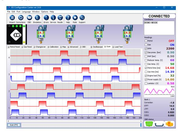
Petrol and gas injection oscilloscope scanner is a tool useful for diagnostic purposes. With use of this scanner it is possible check: the order of the injection sequence, injectors overlapping occurrence, presence of shorts injection pre-pulses etc.
