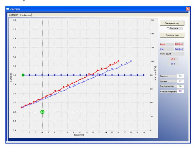
This function makes available to work with **Map** and **Oscilloscope** bookmark maximized to the size of main window. This feature is recommended during collection of petrol and gas map.
