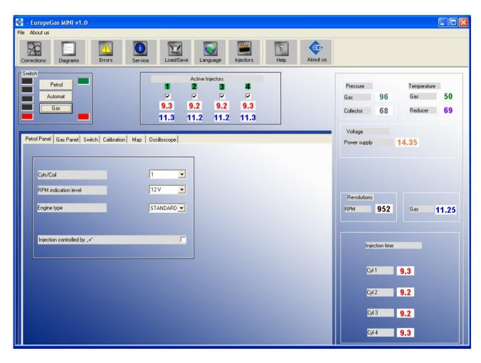
First step after connecting the interface from the computer to OSCAR-N MINI ECU and turning on the program is to set the parameters from the Petrol Panel properly.
