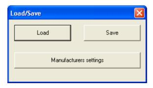
Makes possible to "Save" current program settings in a \*.xset file. All the settings like the multiplier values, sensor types etc. can be saved on disk and easily restored in any moment by pressing the "Load" button. In any moment we can restore original values of the controller by pressing the "Manufacturers settings" button. It is also possible to update the controller's firmware.
