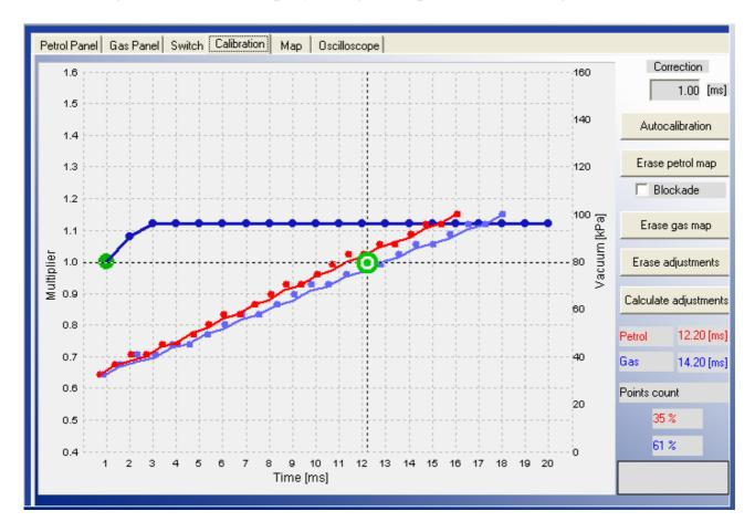
If the injectors nozzle diameter and reducers pressure has been selected properly (which will be confirmed by proper main correction calculated during autocalibration) the petrol and gas map should agree. In case if there are big differences between both lines we can use "Calculate adjustments" option. Gas injectors opening time will be automatically corrected where the distance between both maps (for the same petrol injection opening time) will be too big.
