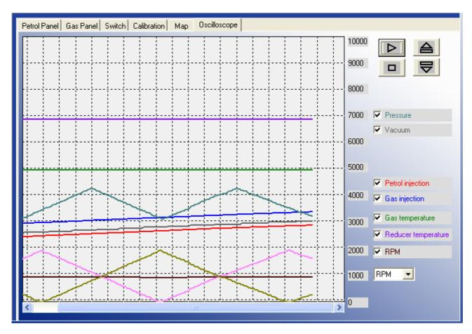
On the right side of this panel we can select which signals measured by the controller we would like to see on oscilloscope and the buttons for Load, Save, Start and Stop the oscilloscope. We can work with following signals:
