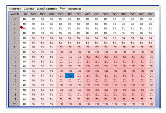
OSCAR-N MINI controller makes possible to adjust the composition of air/fuel mixture in the whole range of engine load. To do this we can use Corrections map placed in the "Map" bookmark (feature protected by password).
