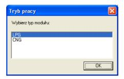
During every start of the software please choose the OSCAR-N MINI ECU work mode **LPG** or **CNG** (depending on the type of installation in the car).
