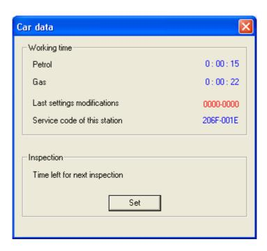
Shows the amount of time that controller has been driving on petrol/gas. Makes possible to set time remaining to the next system inspection. Exceeding that time will be signalized by beeping of the buzzer and switch LED's blinking after each turning on the controller in Auto mode until next system inspection will be set by the installer.
