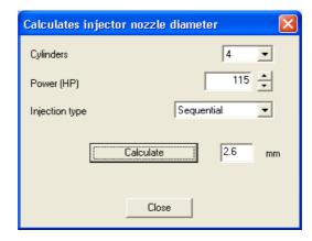
This function makes possible to calculate injection nozzle's diameter according to amount of BHP to one cylinder and injection opening strategy type.
