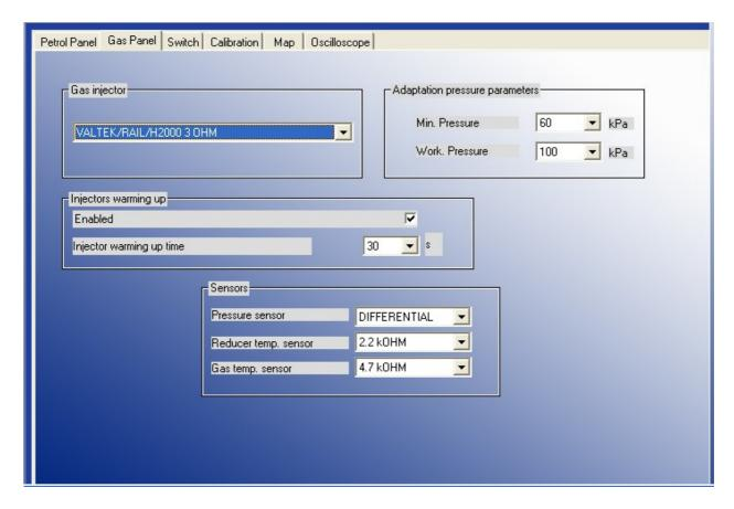
Second step will be selecting the the proper injector rail type (for RAILGAS 3 Ohm injectors please select VALTEK/RAIL/H2000 3 Ohm), and type of sensors from Gas Panel. Selection of wrong sensor will cause improper sensor indication (i.e. wrong selection of gas temp. sensor may cause showing very low reducer temperature on the screen after the start of warm engine)
