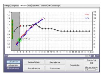
If everything has been installed properly, 4 steps mentioned above should guarantee proper driving on both fuels. In more sophisticated cars there may be necessity of using features located in "Map", "Corrections", Advanced" and "OBD" bookmarks. To learn more details refer to the User's Manual located in "docs" folder attached to the software (Press "Help" bookmark to open that folder).
